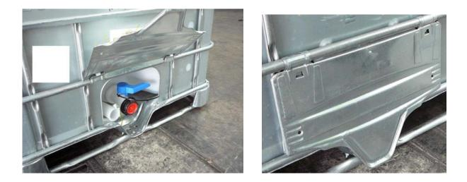
40. Metal IBCs may also fail hydraulically or by ullage space explosion. Consideration could be given to the fitment, whilst in storage, of pressure relief valves to reduce the risk of catastrophic failure in the event of fire. If a third party under contract supplies the IBC, this should be done with their permission and restored to UN specification prior to transport.
